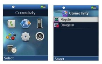
**STEP 21** On the Connectivity dialog and after choosing Register option > Enter the **Access code** (by default is 0000) > Press **OK** > Successful registration displays Extension(s) registered.
