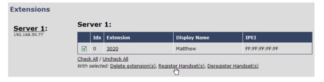
**STEP 20** Next, take the handset you would like to register > power it up > In the idle mode navigate to the Menu > Choose **Connectivity** > Select **Register**.
